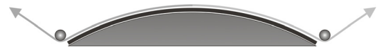
Figure 2: Sketch of the bowed ground plate setup. The wire is mounted in a frame between two springs (marked as arrows). If the wire is pushed to the ground plate, the springs allow the wire the necessary elongation and maintain the wire tension so that the wire snuggles to the solar cell (dark grey).
