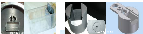
Fig 4. Carrier development for 5 \times 5 \text{ cm}^2 (quartz) and 10 \times 10 \text{ cm}^2 (graphite).
