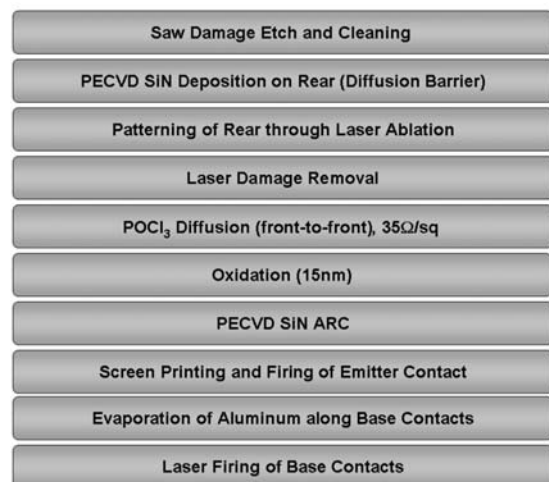
Fig. 2: Processing scheme for IBC cells. Cells were fabricated on 2 Ωcm CZ silicon wafers with an original thickness of 300 μm.
