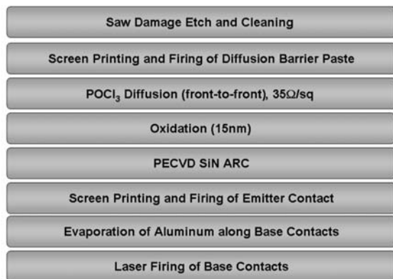
Fig. 8: Simplified processing scheme for manufacture of IBC cells on p-type substrates. Masking of the rear is achieved by the use of a screen printed diffusion barrier paste.
