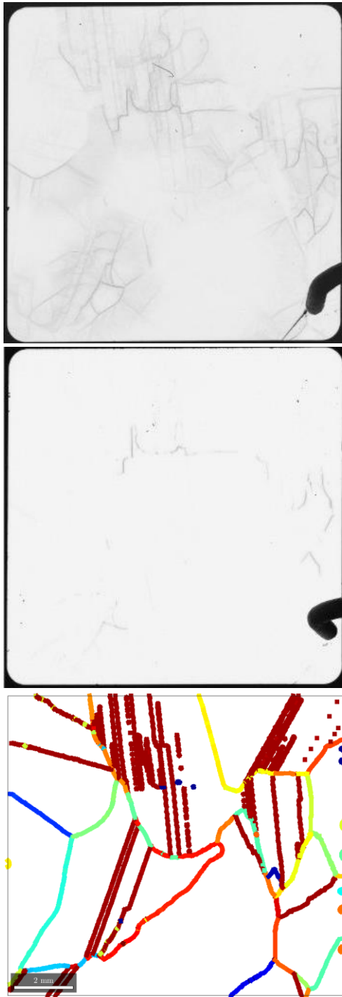
Figure 6: Comparison of EBIC results for the as-grown (top) and APCVD gettered sample (middle) with the misorientation angle between grains at grain boundaries measured via EBSD. The APCVD gettered sample was used for the EBSD measurement.
