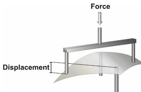
**Figure 1:** Twist geometry used for experiments presented in this paper. The maximum tensile strength and the maximum displacement are measured.
