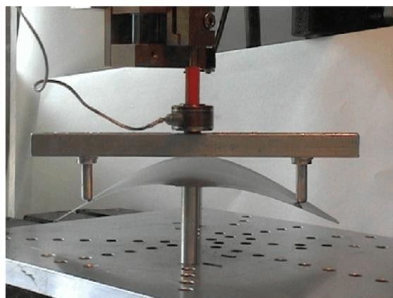
**Figure 2:** Picture of a CZ wafer right before breaking.
