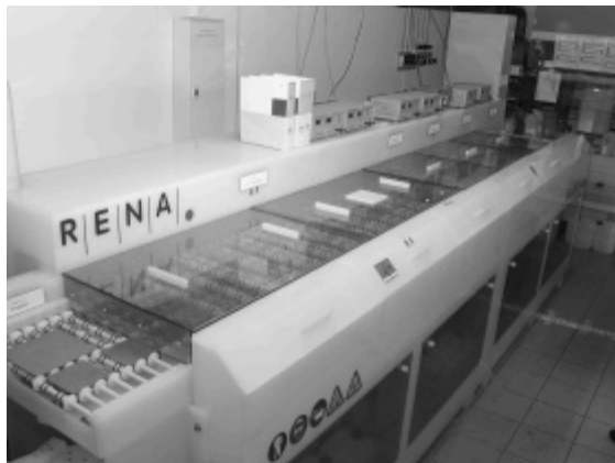
Fig 5: Lab version of the in-line texturing equipment from RENA installed at UKN. On the left lane very large wafers can be processed (left wafer on picture is 200 mm in size).
