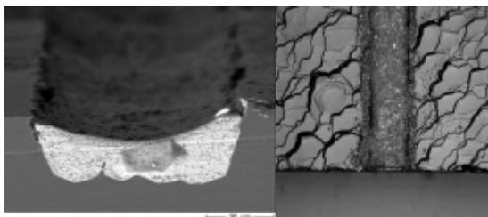
**Fig 1:** Left: SEM picture of groove filled with screen printing paste. Right: Optical microscope top view of a filled groove.
