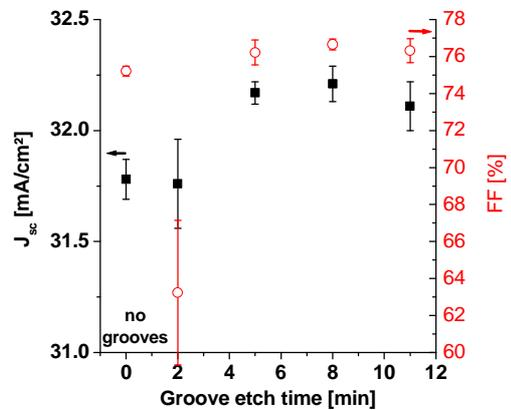
**Fig 5:** Dependence of J<sub>sc</sub> and FF on groove etch time compared to cells without groove.
