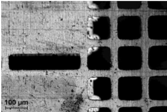
**Fig 3:** Picture of a double layer stencil. The beginning of a finger and part of the busbar are shown. The finger width is 75 μm.
