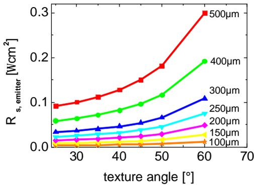
**Figure 3:** Contribution of the emitter on the series resistance versus texture angle for various finger spacings.
