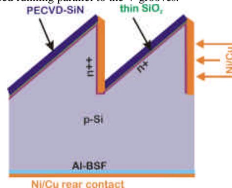
**Figure 1:** Schematic drawing of the EASY & SIMPLE solar cell. The line-shaped contact area is defined mechanically or by directional PECVD.
