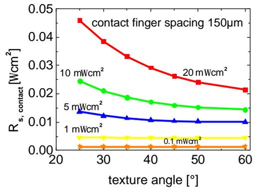
**Figure 5:** The contact resistance for different contact resistivities versus the texture angle. The texture defines the finger width.
