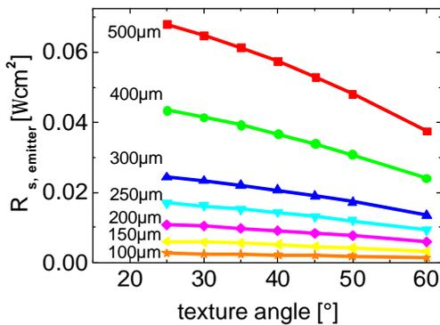
**Figure 4:** Contribution of the emitter to the series resistance versus texture angle for various finger spacings in the case the contact fingers running perpendicular to the texture.
