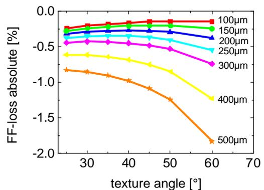
**Figure 6:** The main contribution to the series resistance of the EASY & SIMPLE cells are considered in the FF estimate. The FF-loss absolute is defined as the difference between the ideal FF of 84 % and the calculated one.
