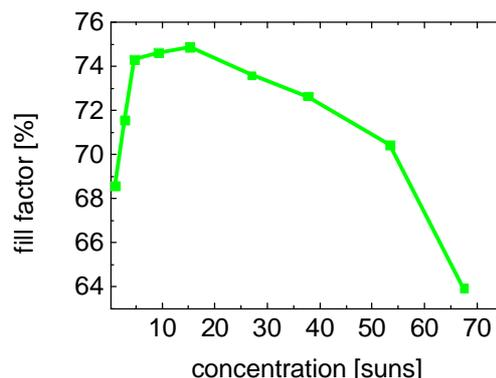
**Figure 8:** Fill factor of an EASY & SIMPLE cell versus light intensity. The high series resistance losses decrease the FF with increasing concentration significantly.
