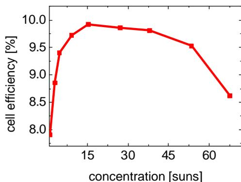
**Figure 7:** Cell efficiency versus light intensity of the first EASY & SIMPLE cells with plated contacts. Maximum efficiency is achieved at 15 suns.
