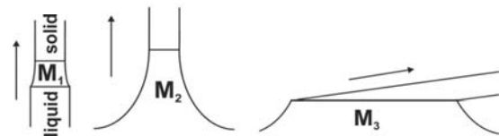
Fig. 1: Shape of meniscus for different ribbon Si techniques.
