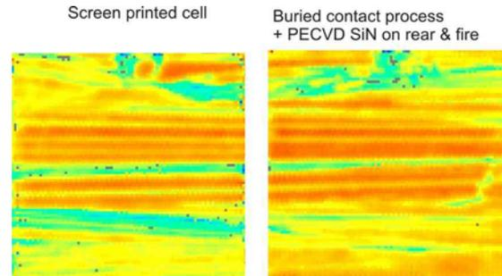
**Figure 10:** Alternativ hydrogen passivation.
