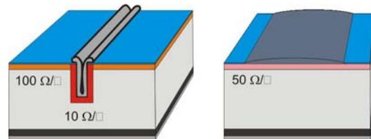
**Figure 1:** Schematic drawing of a buried contact cell on the left side, on the right a screen printed cell.
