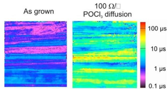
**Figure 4:** Lifetime map of as grown wafer on the left. Improvement after 100 Ohm/sq  $\text{POCl}_3$  diffusion (P-gettering).
