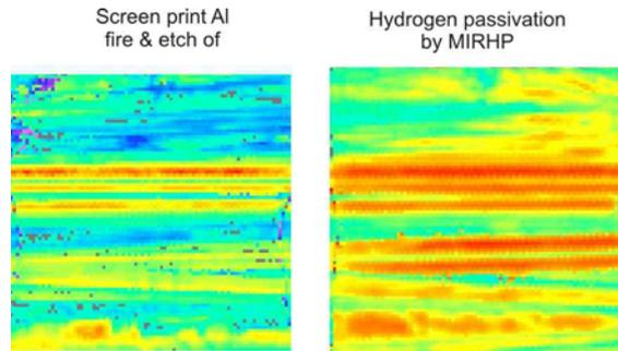
**Figure 8:** Improvement of hydrogen passivation by MIRHP.
