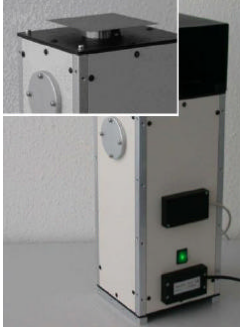
Fig. 6: Photograph of the SPV measurement system for in-line characterization of mc-Si wafers after P-diffusion
