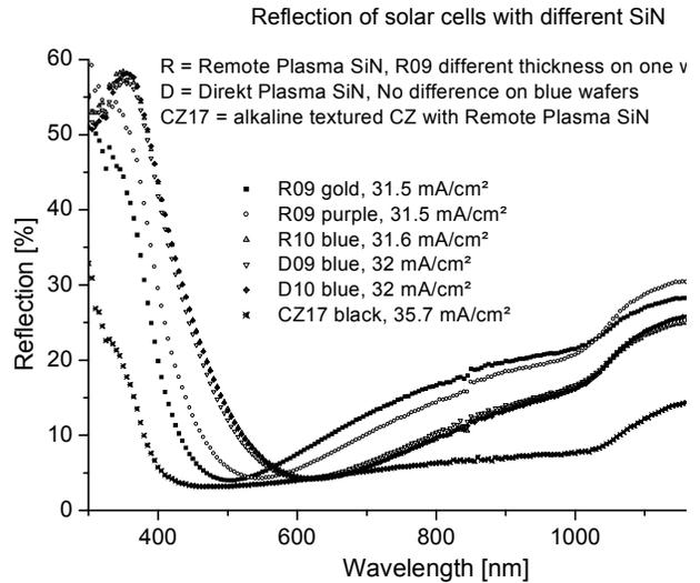
Fig. 5. Reflection of 4 mc and 1 alkaline textured CZ solar cell. Despite the fact that on cell R09 with remote plasma SiN the layer thickness is too thin and the appearance varies from gold to purple there is only a moderate loss in  $J_{sc}$ .
