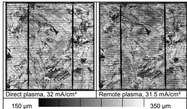
Fig. 6.  $L_{eff}$  mapping of 2 neighbouring wafers with direct/remote PECVD SiN. LBIC mappings with 833, 910 and 980 nm wavelength were used to calculate  $L_{eff}$ .
