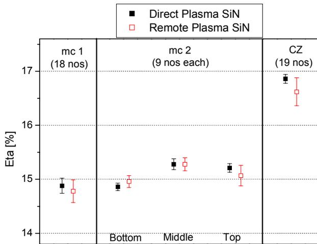
Fig. 4 Mean values and deviation of efficiency of solar cells with direct/remote PECVD SiN. Only on CZ Si direct plasma SiN leads to better results.
