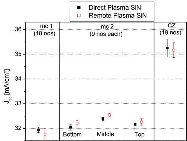
Fig. 2 Mean values and deviation of short circuit density  $J_{sc}$  of solar cells with direct/remote PECVD SiN.
