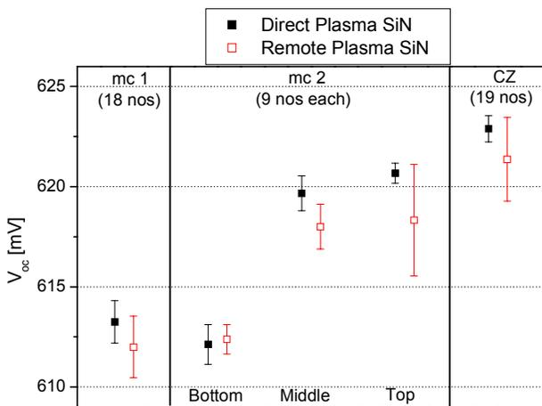
Fig. 1 Mean values and deviation of open circuit voltage  $V_{oc}$  of solar cells with direct/remote PECVD SiN. On good quality material with high  $V_{oc}$  the direct plasma SiN is superior.
