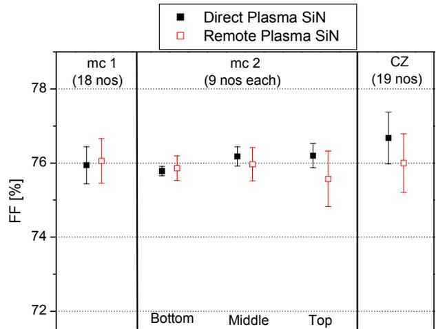
Fig. 3 Mean values and deviation of fill factor FF of solar cells with direct/remote PECVD SiN. No significant difference can be seen.
