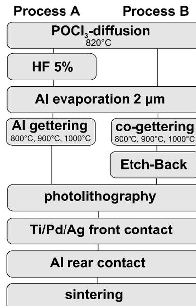
**Figure 1:** Solar cell process for Al-gettering (Process A) and P-Al co-gettering (Process B).
