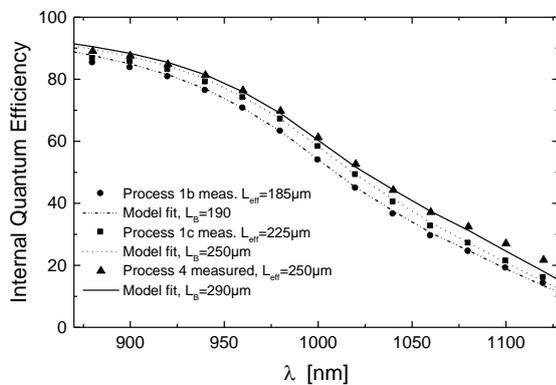
**Figure 4:** Model data (lines) calculated with PC1D and measured data (points) for best cells of Process 1b, 1c and 4.  $L_{\text{eff}}$  was obtained from a spectral analysis of the measured curve,  $L_{\text{B}}$  was used in PC1D for the model calculation.
