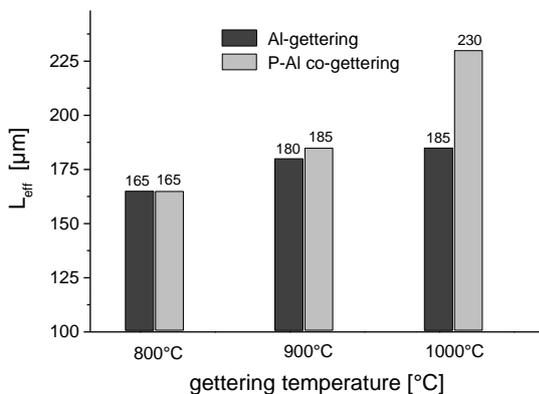
**Figure 2:** Effective diffusion lengths  $L_{eff}$  obtained from a spectral analysis of the IQE in the infrared of Al-gettered (Process A) and P-Al co-gettered (Process B) cells for different gettering temperatures. Given are average values of four cells.
