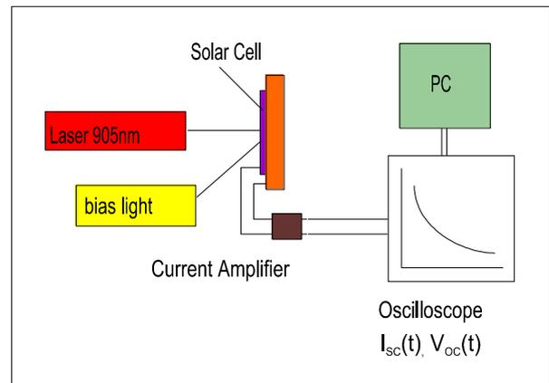
**Fig. 2:** The experimental setup of the PCVD-measurement.
