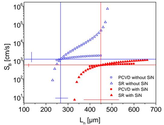
**Fig. 5:** Parameter plots  $S_B(L_n)$  for two solar cells with and without a fired silicon nitride (SiN) ARC. The cells are made of CZ-material. A large increase of the diffusion length is clearly visible.
