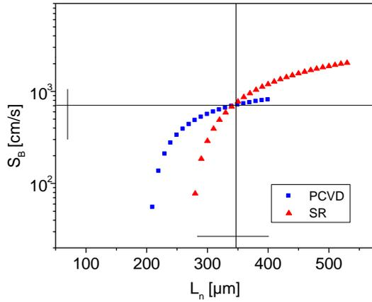
**Fig. 3:** The parameter-plots  $S_B(L_n)$  from the  $\tau_j$  (PCVD) and the  $L_{eff}$  (SR). The point of intersection supplies  $L_n$  and  $S_B$ . The bars parallel to the graph axis give the uncertainty of the measurement.
