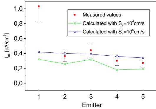
**Fig. 9:** The measured saturation currents of the five emitters compared with calculated values. The calculations were done for  $S_F = 10^4$  and  $10^5$  cm/s with the program PC1D.
