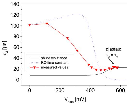
**Fig. 4:**  $\tau_U$  in dependence on the cell-voltage due to the bias light. Further the influence of the capacitive time constant of the pn-junction and the shunt resistance of the cell are shown (explanation in the text).
