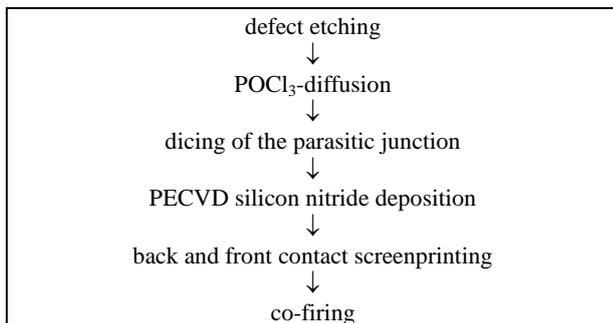
**Fig. 1:** The process sequence of screenprinted solar cells. The front metallization is fired through the silicon nitride in the final co-firing step.
