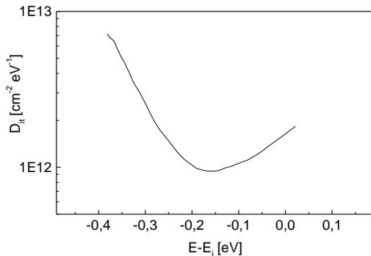
Fig. 12: The interface trap density  $D_{it}$  of a PECVD silicon nitride MIS-sample in dependence of the energy in the bandgap. The SiN was deposited at 305°C 780  $\text{W/m}^2$  and fired in an infrared furnace. The midgap  $D_{it} = 1,2 \cdot 10^{12} \text{ cm}^{-2} \text{ eV}^{-1}$  and the fixed charge  $Q_{SS} = 3,2 \cdot 10^{12} \text{ cm}^{-2}$ .
