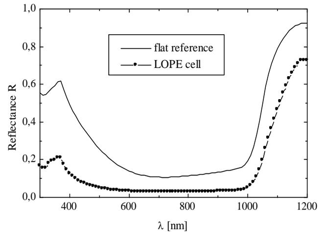
**Fig. 7:** Hemispherical reflectance  $R$  of a LOPE solar cell in comparison to a flat reference cell with the same single layer ARC and local BSF.
