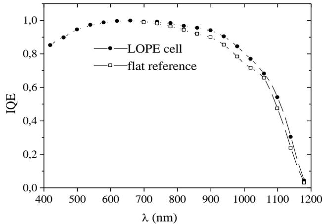
**Fig. 8:** IQE of a LOPE cell and a flat reference (because of technical problems the reference could not be measured over the whole range)
