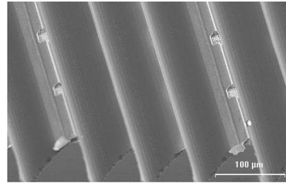
**Fig. 3:** SEM picture of local point contacts on the V-groove tops of a LOPE cell. The fingers, evaporated under a shallow angle, which are interconnecting the single point contacts, are visible at the V-groove tips (V-groove sequence 3, see text).
