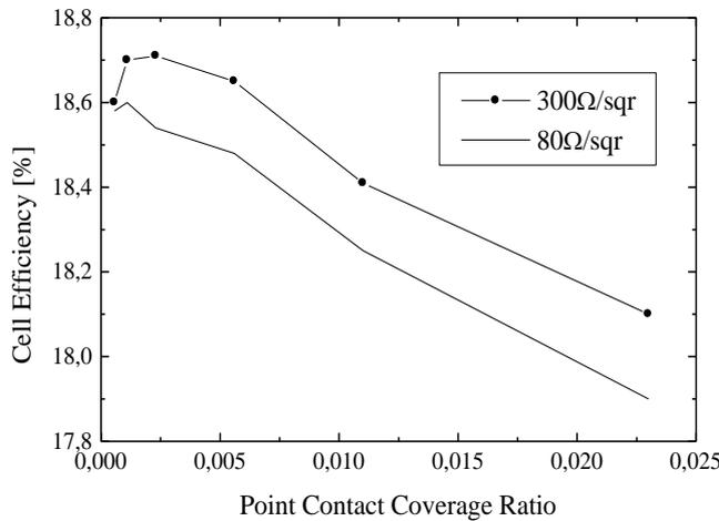
**Fig. 5:** Optimisation of local point contact distances and comparison of two different shallow emitters ( $L_D=200\mu\text{m}$ , full BSF).
