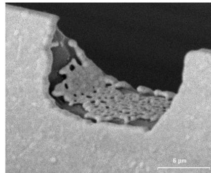
**Fig. 4:** SEM picture of a single local point contact, which was metallized using the shallow angle evaporation. The width of the point contact openings is approximately  $15\mu\text{m}$ .
