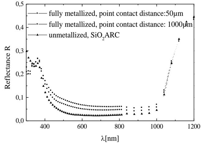
**Fig. 6:** Hemispherical reflectance  $R$  of a LOPE solar cell with different point contact distances compared to an unmetallized LOPE cell. All LOPE cells have got an anti-reflection coating, ARC, of  $\text{SiO}_2$  and full Al BSF.
