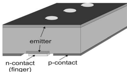
Figure 5: The EWT cell design has both emitter and base contact on the rear side of the cell, requiring interdigitation. The emitter contact is connected to the frontside emitter through metallised, laser drilled holes.
