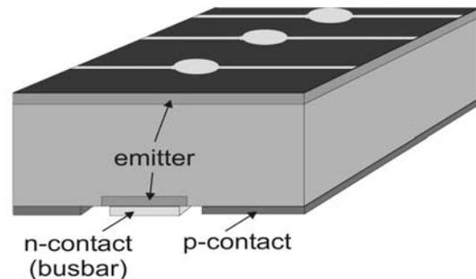
Figure 3: Schematic of a MWT solar cell. The frontside emitter contact finger grid is connected to the emitter busbars, located on the rear side of the wafer, through metallised holes. The design allows for a multiple busbar design without increasing shadowing losses.
