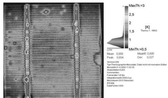
Figure 4: Thermographic image of a MWT solar cell. The cell shows shunting along the emitter busbars located on the rear surface of the cell if the same ink is used for frontside finger grid and rear side busbars. This is the major loss mechanism at the current stage of our cell development.
