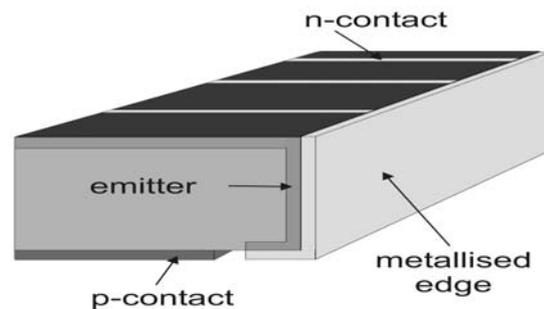
Figure 1: Schematic illustration of a Metallisation Wrap Around solar cell. The front fingers are connected to the emitter contact on the rear over two opposite edges. External p- and n-contact isolation was realised by isolating trenches.
