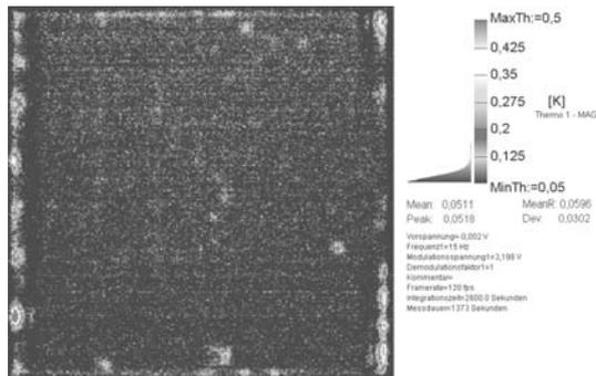
Figure 2: Thermographic image of a MWT solar cell. The lighter areas represent local shunts at the metallised edges, limiting fill factors and cell performance.
