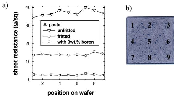
**Figure 2:** a) Sheet resistance depending on paste and position on the Si-wafer (25 cm<sup>2</sup>). b) Picture defining the different positions.
