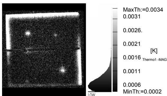
**Figure 4:** IR-thermography after insufficient edge isolation. Especially the top edge is completely shunted because of a  $p^+n^+$  short circuit transition.
