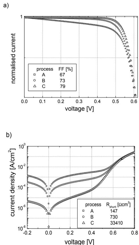
**Figure 3:** a) Illuminated and b) dark IV-characteristics for different processing sequences A, B and C.
