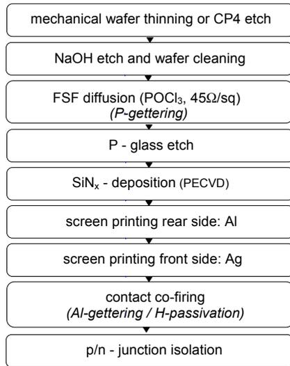
**Figure 1:** Basic process sequence of our standard back junction solar cell.
