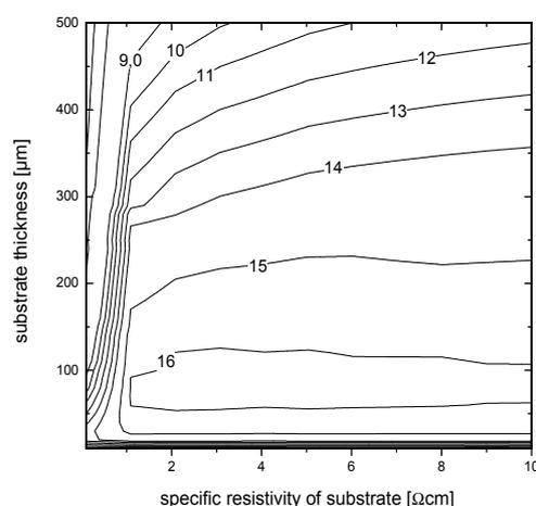
**Figure 5:** Efficiency dependence on substrate thickness and specific resistivity.
