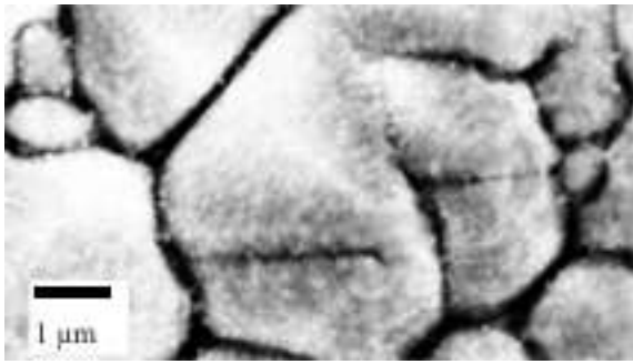
Figure 14: SEM surface analysis of a sample with a starting sheet resistivity of 50 Ω/sq. A structural change of the pyramid surface becomes visible.
