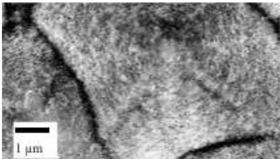
Figure 16: SEM surface analysis of a sample with a starting sheet resistivity of 120 Ω/sq. A high morphological change of the surface can be observed.
