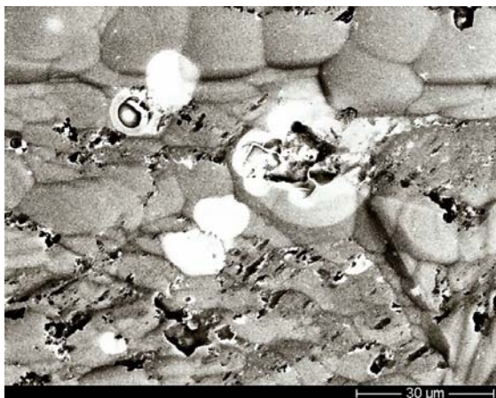
Figure 2: Electron microscopy of the shunted part of the wafer shown in Figure 1 (left). EDX scans of this region (Figure 3) identified the shown formations as aluminium.
