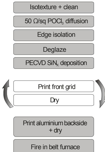
**Figure 3:** Process sequence used for the “built up” solar cells. It is a standard screen print solar cell process except for the repeated front grid printing and drying.
