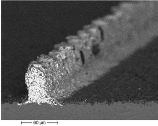
**Figure 5:** SEM image of ten-fold printed finger after firing (60 $\mu$ m width, 60  $\mu$ m height).
