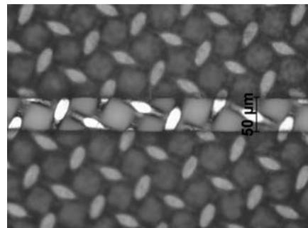
**Figure 2:** Optical microscope image of modified screen. Finger opening is only 50  $\mu\text{m}$  wide. Outside the opening, the mesh is covered with the emulsion layer. The mesh is calendared, visible at the flattened crossing points of the wires.
