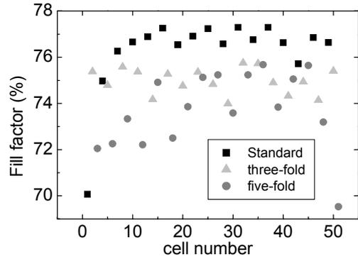
**Figure 7:** Fill factors as a function of cell number. Standard screen printed cells had higher fill factors compared to the three-fold and five-fold printed cells. Cell 1 and 51 were neglected in the analysis due to exceptionally low fill factors.
