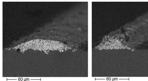
**Figure 4:** SEM images. Left: Standard screen printed finger (120μm width, ~15 μm height). Right: three-fold printed finger (60μm width, ~25 μm height).
