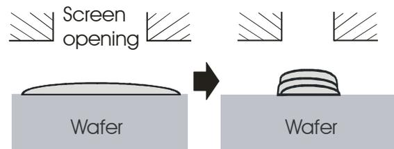
**Figure 1:** Left: Cross section of a standard screen printed finger (typical screen opening: 100  $\mu\text{m}$ , finger width 120-140  $\mu\text{m}$ ). Right: Cross section of a triple stack finger, made by printing three times with intermediate drying. Thinner fingers can be printed using a modified screen.
