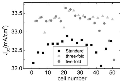
**Figure 6:** Short circuit current values of all cells. Three-fold and five-fold printed cells show higher  $J_{sc}$  values due to lower shading losses.
