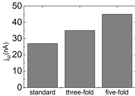
**Figure 7:**  $j_{02}$  values obtained by fitting the illuminated IV-curves to a two diode model: mean values.
