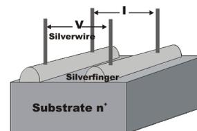
**Figure 2:** Experimental setup of the in-situ  $R_c$  measurement
