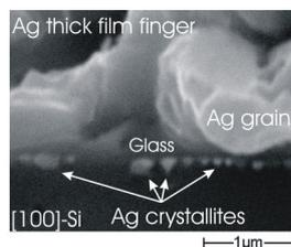
**Figure 1:** SEM-picture of the interface of a silver thick film finger on [100]-orientated silicon.
