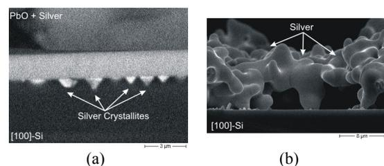
**Figure 8:** SEM cross section pictures: (a) PbO+Ag on [100] silicon. (b) pure Ag on [100] silicon.
