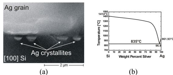
**Figure 4:** (a) SEM cross section picture of silver on [100]-orientated silicon after firing at  $900^\circ\text{C}$  for 15 min. (b) Silver-Silicon phase diagram (after [1]).
