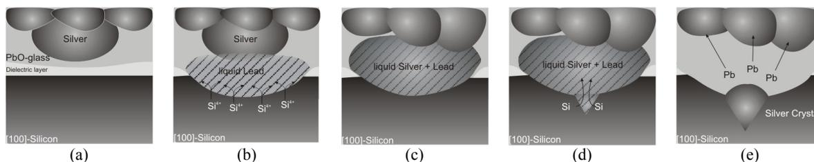
**Figure 9:** Silver growth model. (a) Schematic cross section of Ag thick film paste on [100] silicon after burn-out. (b) Glass has penetrated the dielectric layer → redox reaction between glass and silicon. (c) Silver particle dissolves in liquid lead according to phase diagram. (d) Silicon interacts with liquid silver – lead alloy → formation of inverted pyramids. (e) Phase separation on cooling down → Silver recrystallizes on [111] planes of the pyramid.
