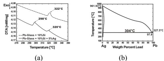
**Figure 7:** (a) DTA measurement: Second heating cycle of different mixtures. (b) Silver – Lead phase diagram (after [1]).
