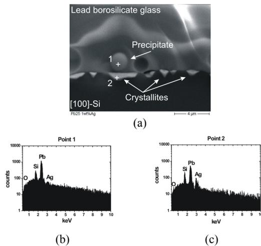
**Figure 5:** (a) SEM cross section of paste 1 on [100] silicon. (b) EDX analysis of point 1. (c) EDX analysis of point 2.
