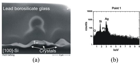
**Figure 6:** (a) SEM cross section picture of paste 2 on [100] silicon. (b) EDX analysis of point 1.
