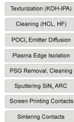
Figure 1: Scheme of cell processing steps
