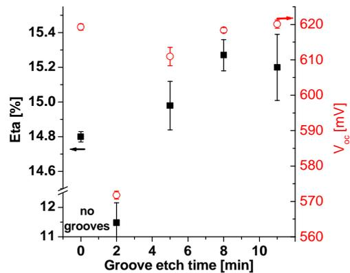
**Fig 6:** Dependence of η and V<sub>oc</sub> on groove etch time compared to cells without groove.
