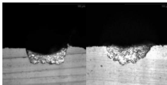
**Fig 2:** Different groove shapes filled with screen printing paste.
