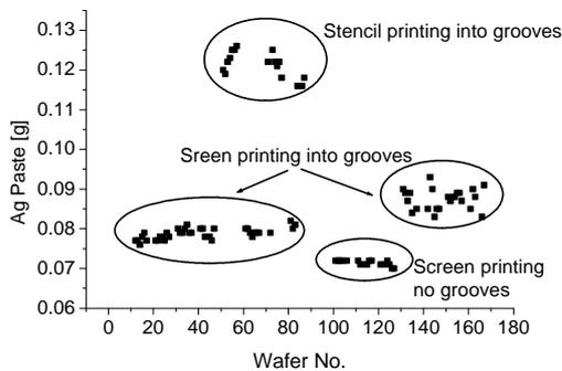
**Fig 4:** Paste weight after printing and drying for different printing methods. For both screen printing methods the same screen was used.
