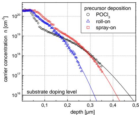
**Figure 2:** ECV profiles of POCl<sub>3</sub>-, roll-on and spray-on emitter diffused at ~ 900°C
