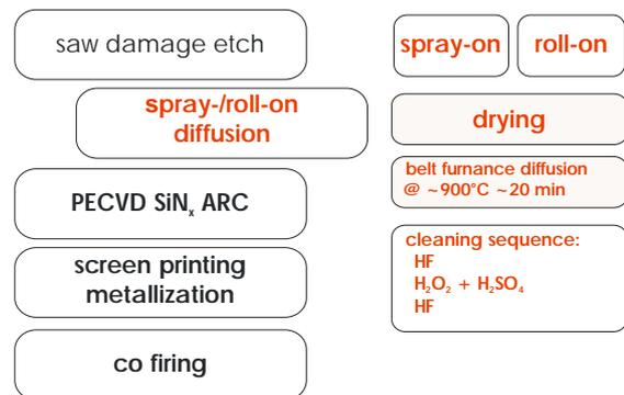
**Figure 1:** Solar cell process sequence using spray- or roll-on precursor deposition
