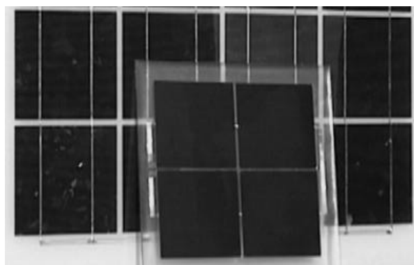
Fig. 7. Photo of a mini-module made of 4 back-contact cells (Cz) in front of a module of conventional cells. The back-contact cells can be arranged with nearly no space between them. The homogeneous optical appearance is very appealing compared to the conventional cells with the reflecting busbars. The mini-module was IV-measured at ECN, Netherlands, with J_{\text{sc}} = 3.62 A, V_{\text{oc}} = 2.39 V and an efficiency of 14.0 %.
