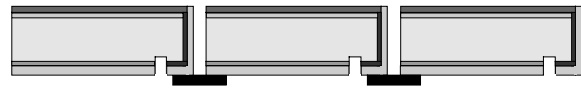
Fig. 3: Cell arrangement of MWA solar cells with one wrap around contact in a module. With this arrangement the I^2R power losses of the cell interconnection can be reduced.
