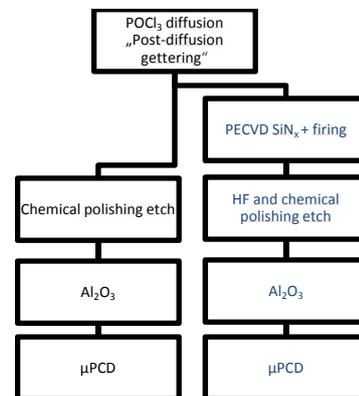
**Figure 2:** Experimental sequence of lifetime measurements.
