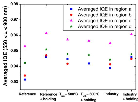
**Figure 15:** Averaged IQE within wavelength interval  $550 < \lambda < 900$  nm versus type of diffusion.
