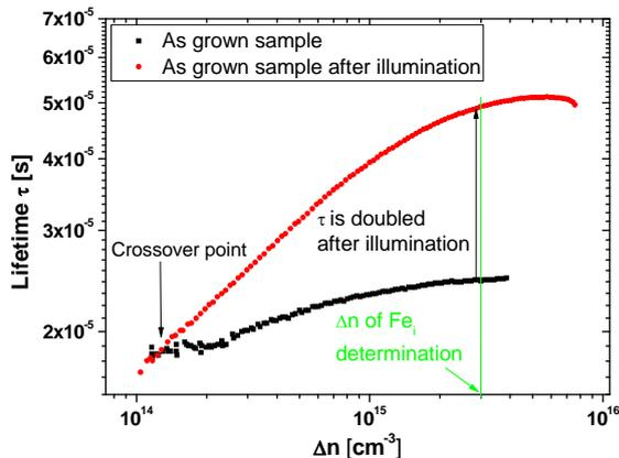
**Figure 3:** QSSPC lifetime before and after illumination of an as grown sample.
