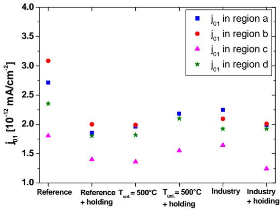
**Figure 14:** Saturation current density  $j_{01}$  versus type of diffusion.
