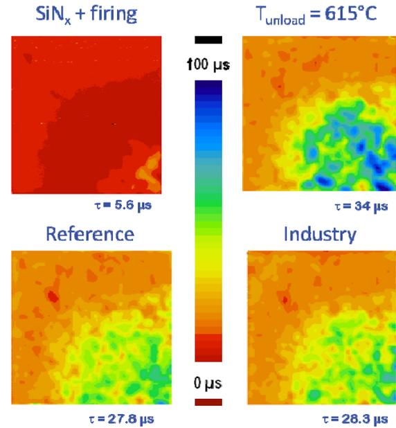
**Figure 7:** Same as in Figure 5 with an additional SiN<sub>x</sub> deposition and firing step.
