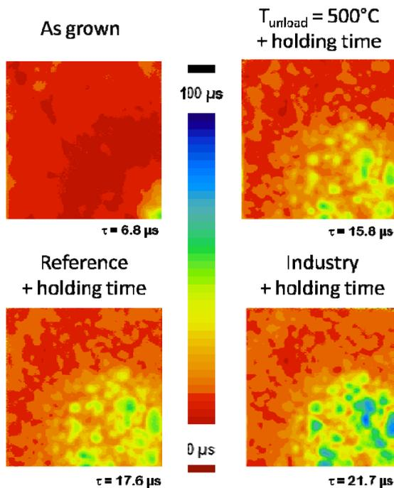
**Figure 6:** Same comparison as in Fig. 5 except that diffusion processes include a holding step at the respective unloading temperature.
