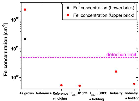
**Figure 9:** Determination of  $\text{Fe}_i$  concentration before and after Phosphorus gettering.  $\text{Fe}_i$  concentrations of gettered samples are below detection limit.
