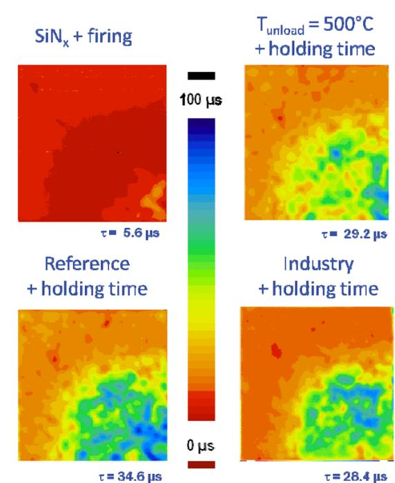
**Figure 8:** Same as in Figure 6 with an additional SiN<sub>x</sub> deposition and firing step.
