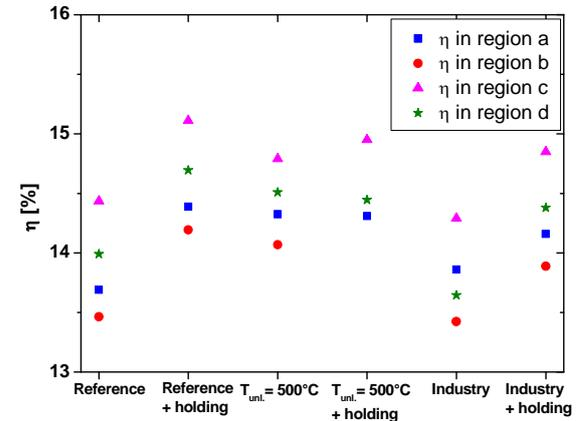
**Figure 11:** Efficiencies  $\eta$  versus six diffusion processes summarized in Table I. Each color resembles one of the different wafer regions a, b, c and d.
