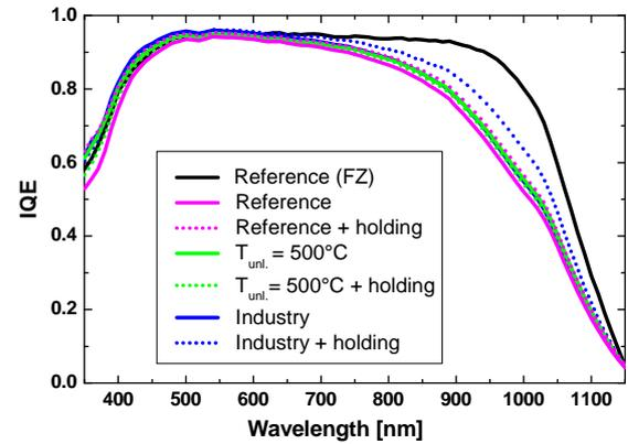
**Figure 17:** IQEs vs. wavelength shown for mc wafers with different emitters. For comparison one FZ cell with reference emitter is added in black.
