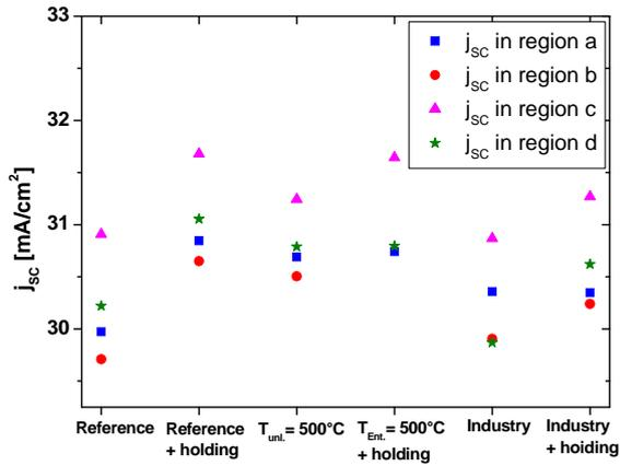
**Figure 13:** Short circuit current density  $j_{sc}$  versus type of diffusion.
