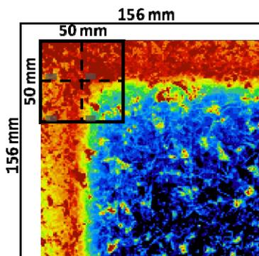
**Figure 1:**  $5 \times 5 \text{ cm}^2$  wafers under investigation are selected out of a  $156 \times 156 \text{ mm}^2$  mc wafer. (Red: low lifetimes; blue: high lifetimes)
