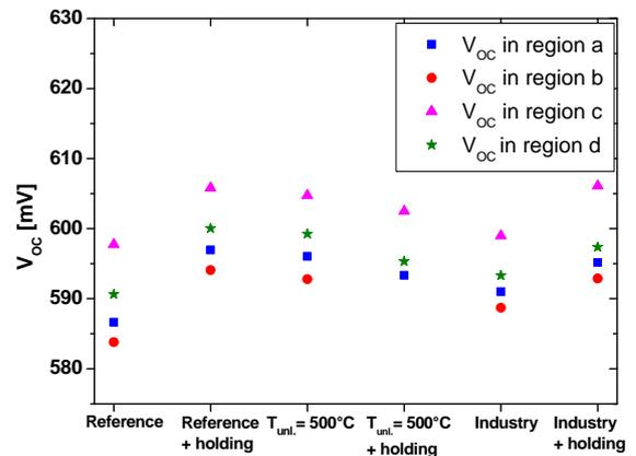
**Figure 12:** Open circuit voltage  $V_{\text{OC}}$  versus type of diffusion.
