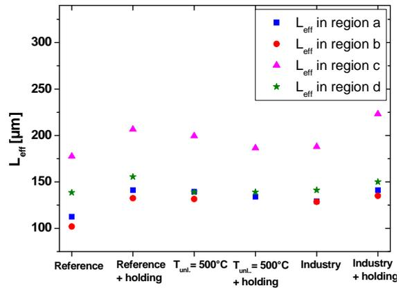
**Figure 16:**  $L_{eff}$  versus type of diffusion.
