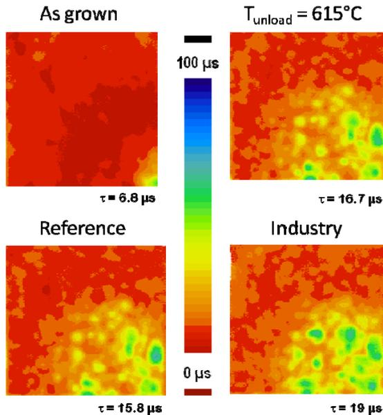
**Figure 5:**  $\mu\text{PCD}$  lifetime comparison of an as grown mc wafer with three sister wafers that are diffused in three different diffusion processes. Given are the mean  $\tau$  values.
