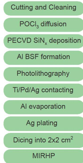
**Figure 4:** High efficiency cell process for mc wafers.
