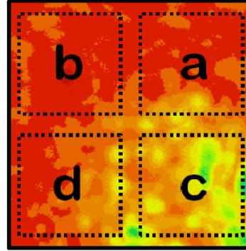
**Figure 10:** Positions of four cells onto a  $5 \times 5 \text{ cm}^2$  wafer. Area c can be identified as the best cell material.
