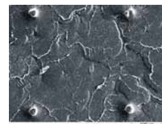
Figure 13b: Top view, after removal of the Al-Si. The unalloyed regions are visible as towers protruding from the surface.
