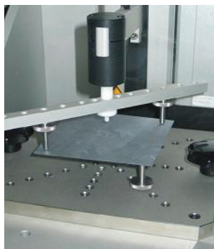
Figure 4: Commercially available STAB-TEST system used for stability characterization by twist testing.
