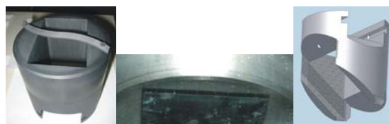
Figure 6: stirrer/ horizontal wafer in carrier/ latest carrier
