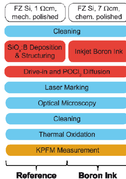
Figure 1: Sample preparation for the reference and the boron-containing ink process.
